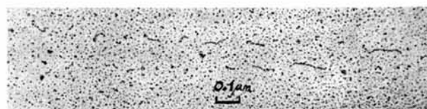
Fig. 8. Linear aggregation of iron nuclei on potassium iodide surface vacuum-cleaved and air-exposed at room temperature.
