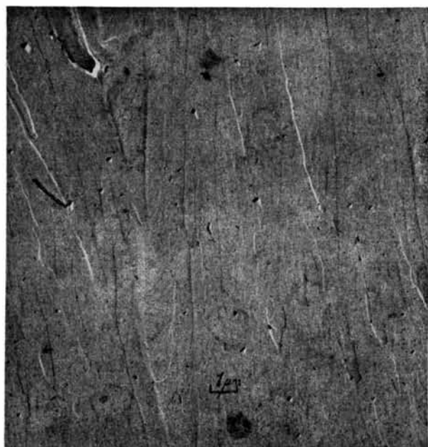
Fig. 4. Iron deposit on potassium iodide surface cleaved during deposition at 300 \text{ \AA} \cdot \text{min}^{-1} . Substrate temperature 120°C.
